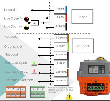
Standard Modulating including Failsafe and Hi-Speed Wiring: Additional wiring options available online.
